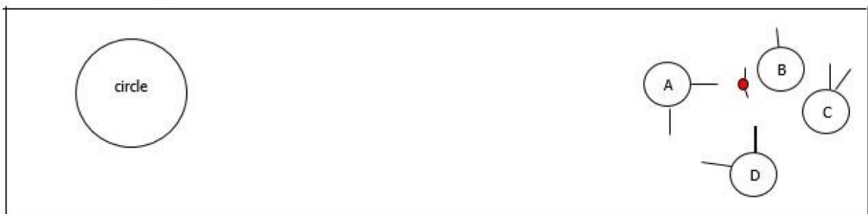
Fig 2b (Incorrect markings) A = faces the jack; B = only 1 line; C = not at right angles; D = one line faces the circle and one is too thick; ● = parallel lines so no cross is able to be made
